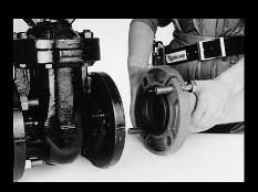
Stretch the gasket around the pipe end and press it into the cavity between the pipe OD and the Quikflange™. The gasket is properly inserted when the sealing lips face the pipe end and the mating flange. The part of the gasket in contact with the pipe should not protrude over the end of the pipe. Apply additional Quikcoup 27-XL lubricant to the outer lip which seals the mating flange.
