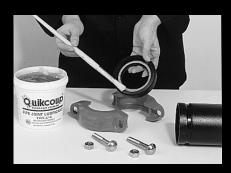
Check the color code of gasket to make sure it is the correct type for service intended. Coat with a thin layer of QUIKCOUP 27-XL lubricant the gasket lips, gasket exterior. (CAUTION: Guard lubricant surfaces against dirt setting on them.)
