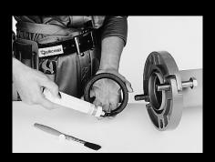
Check the color code of gasket to make sure it is the correct type for service intended.
