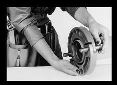
Insert standard bolt through mating bolt holes opposite the hinge to ensure that the Quikflange™ rests firmly in the groove.
